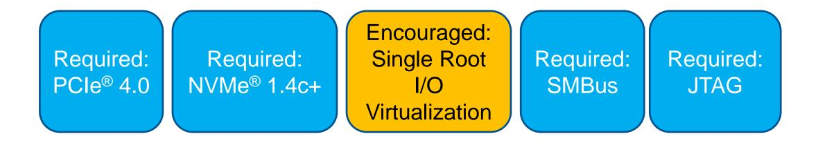
Physical interface Logical interface Optional virtualization System and power management Testability
